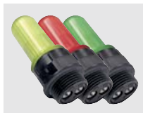
Light indicators A light indicator is used in order to visualize a change of state of the electric contacts inside the switch. It can be installed only in the series FL, FX, FZ or FS by screwing it on one of the conduit entries not used for electric cables. Protection degree IP67.
