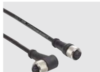
Female connector M8 and M12 - Self-locking vibration-damping ring nut. - High flexibility wire suitable to be used in movable chains - Protection degree IP68 - Gold plated contact (resistance < 5 mΩ) - Connector body in polyurethane
